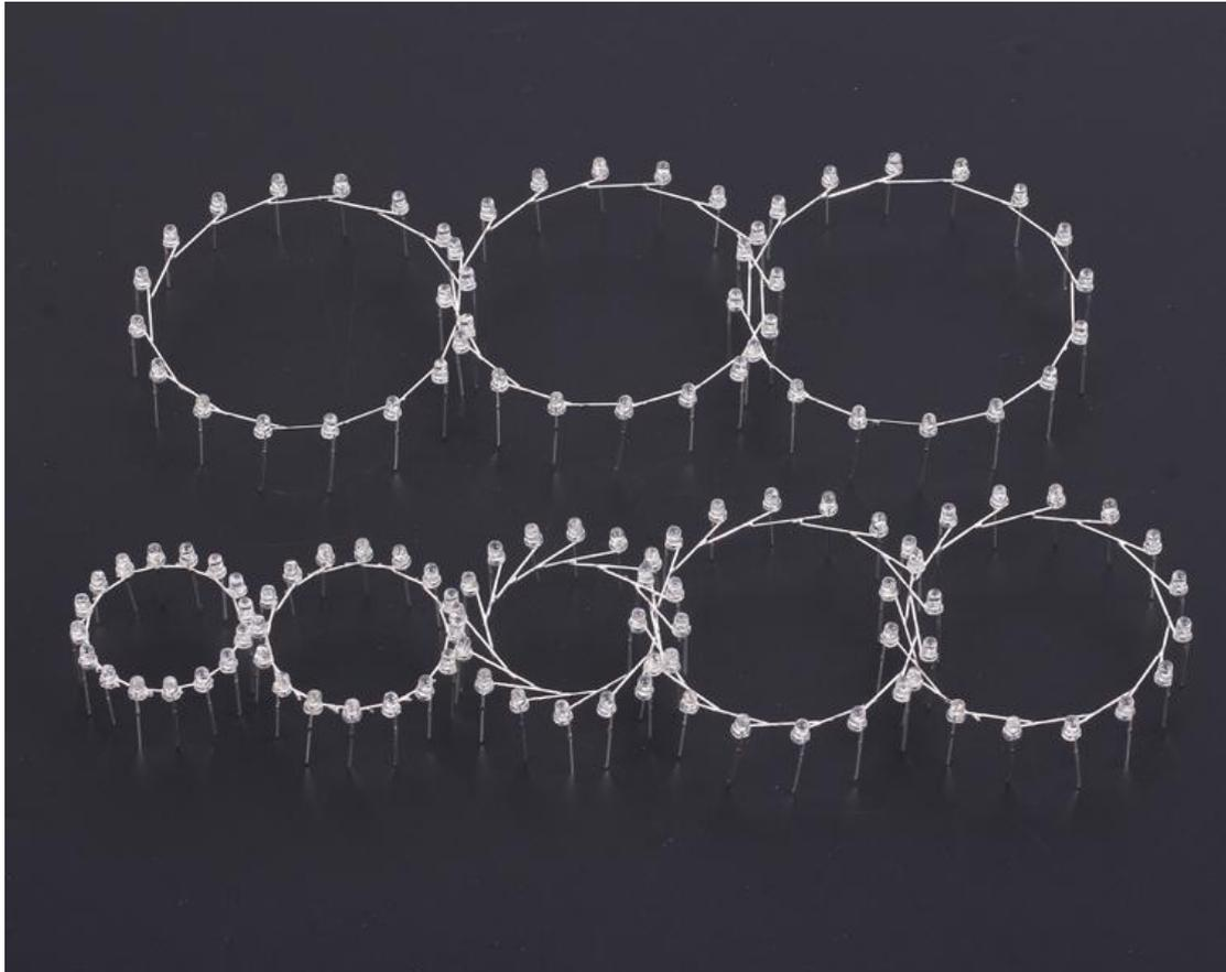
Step 12: Install the 6th Ring as the 1st Layer LED.Bend the pins slightly.First fix a pin, and then fixed the pin on opposite position.Use pliers to bend the tip of the pin if not convenient to install.
