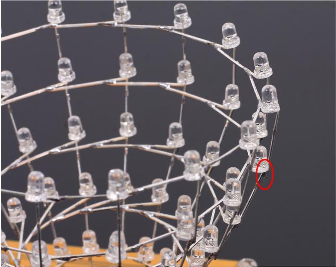
Step 14: Install 6th~8th layer, but bend the LED pins in different ways.
