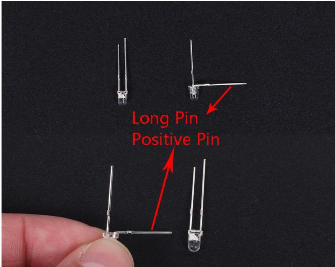
Step 10: Install the 1st Ring LED with Acrylic welding template. Short pin(Negative pole) outward, Longer pin(Positive pole) interconnection.
